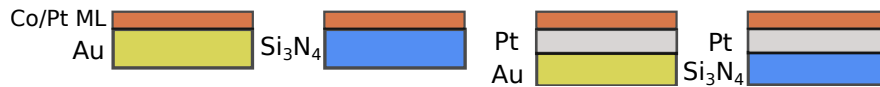
Figure 5.1: In the picture samples analysed in this chapter are schematically depicted. The same Co/Pt ML of thickness 8.8 nm is grown on different substrates. Each colour represents a material, as indicated in the figure.
