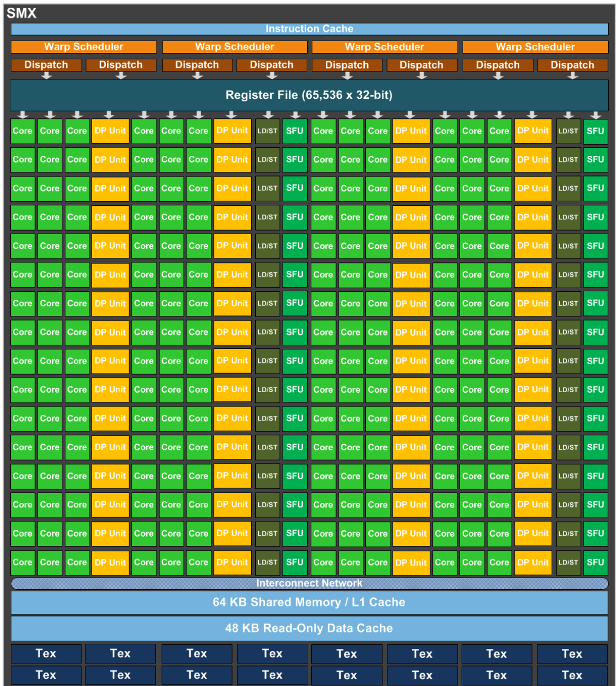
Figure 2.8: A NVIDIA Kepler Streaming Multiprocessor: 192 single-precision CUDA cores, 64 double-precision (DP) units, 32 special function units (SFU), and 32 load/store units (LD/ST).
