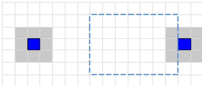
**Figure 3.19: new DT (blue) and 8 pixels around it. If at least one window sits in at least one of these 8 pixels, the new DT can be added to a window.**
