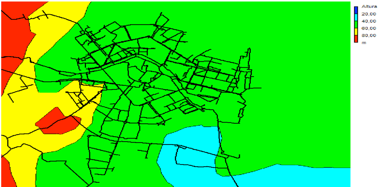
Fig.5.40:Map of isolines of piezometric heads at 12:00 pm in the day of the charging state
