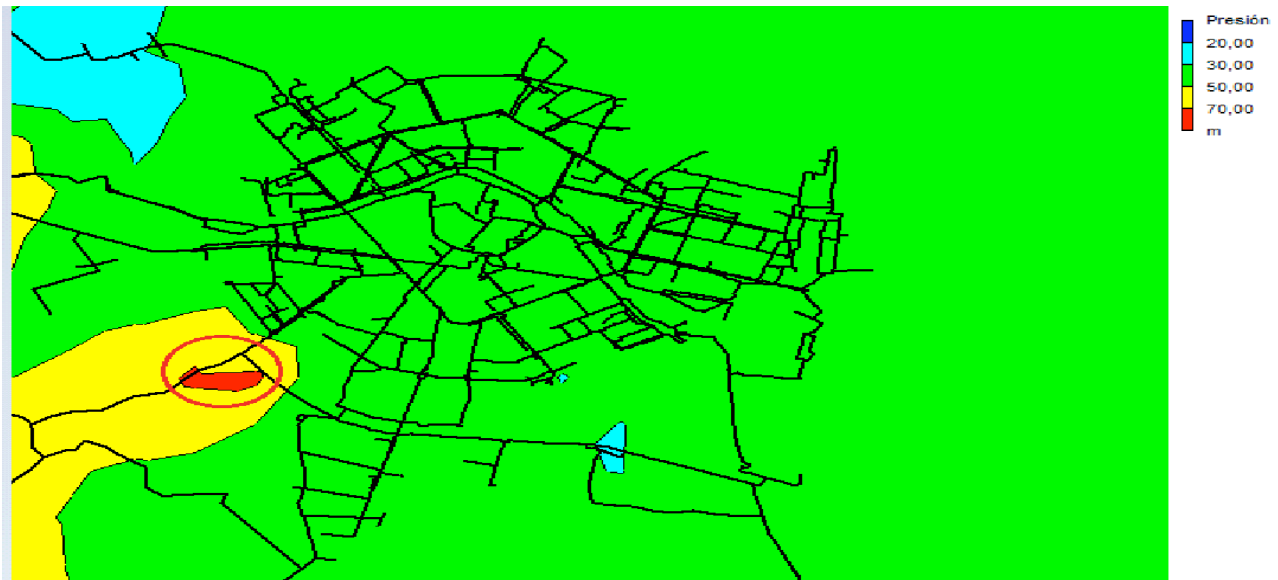
Fig.5.51:Map of isolines of pressure of the network at 07:00 am
