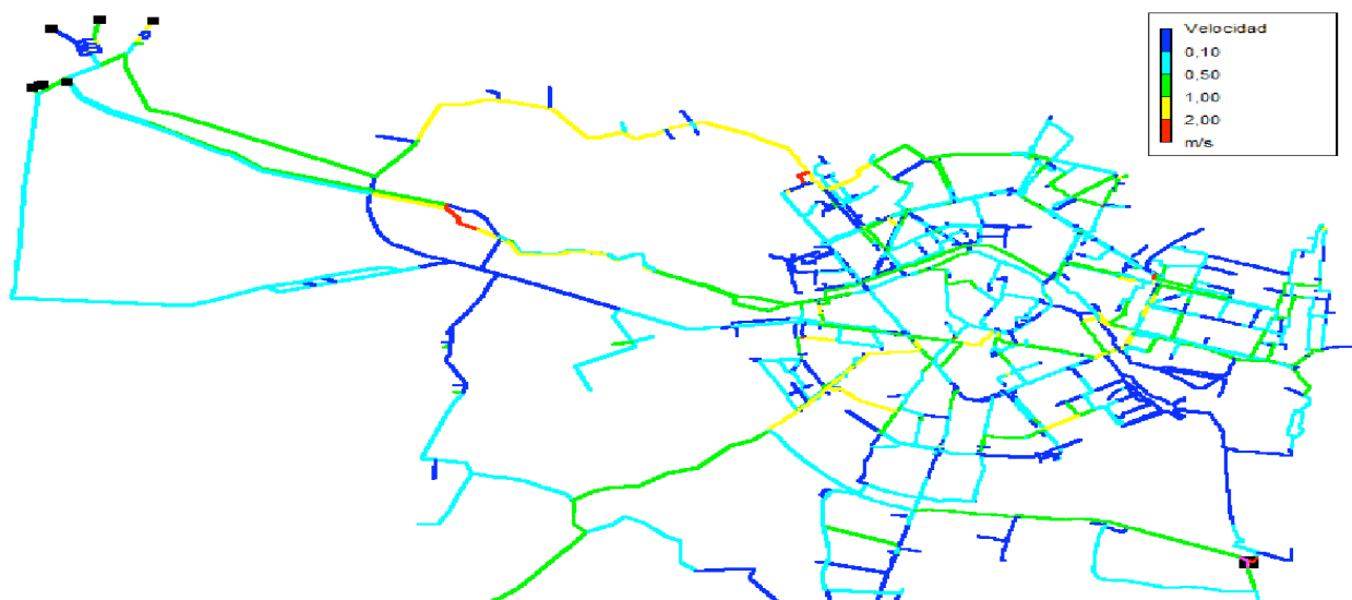
Fig.5.20: Circulation speeds in the pipes at 12:00 pm in the day of the charging state
