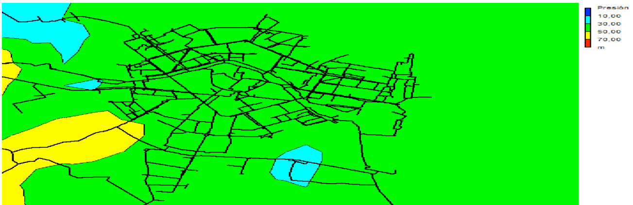
Fig.5.34:Map of isolines of pressure at 12:00 pm in the day of the charging state
