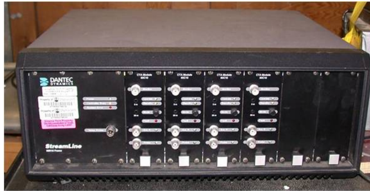
Figure 4.6: Dantec Hot-Wire CTA control circuit.
