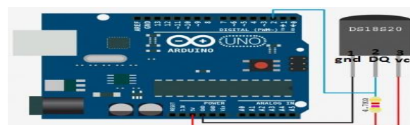
Fig. 3. Connection of temperature sensor to Arduino
