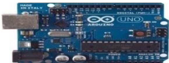
Fig. 1. Microcontroller board of Arduino UNO R3
