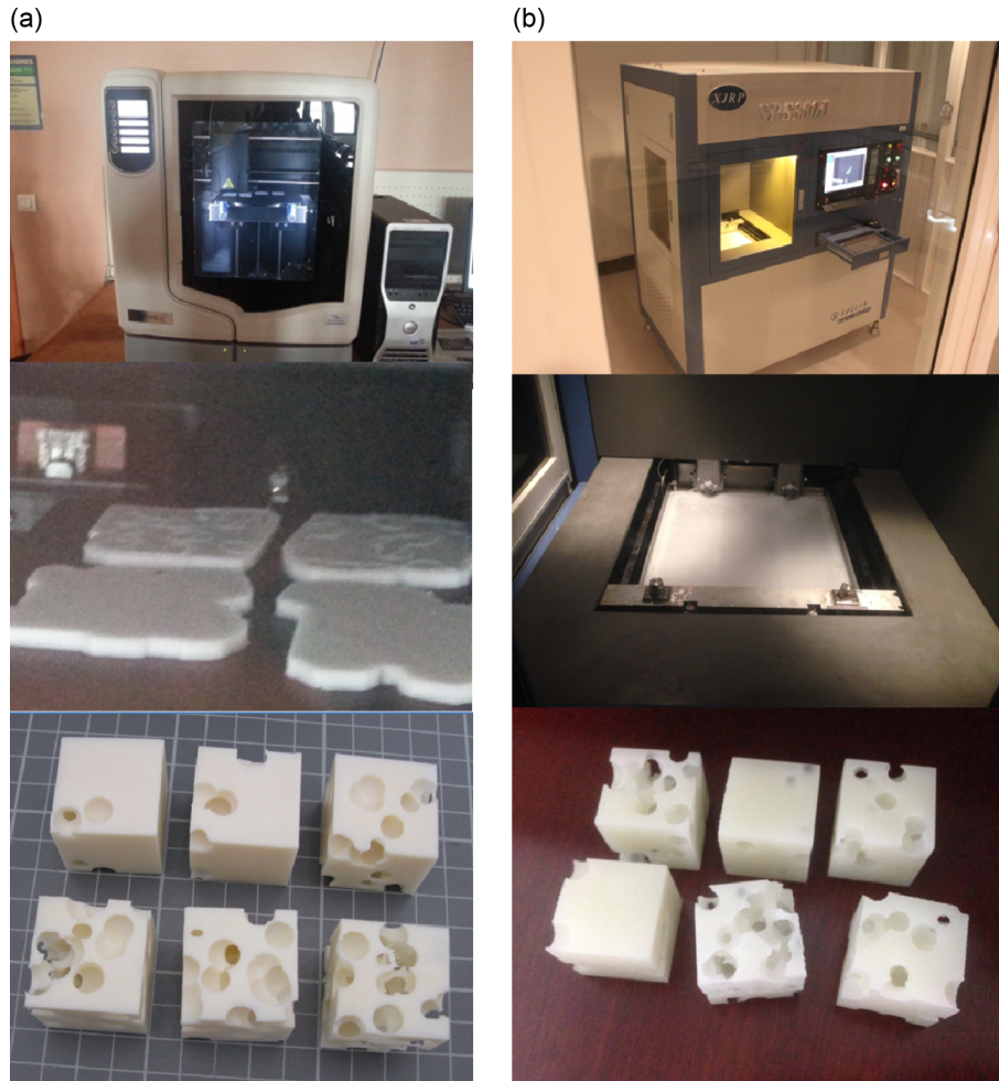
Figure 4. Two examples of airy randomly structured polymers designed using (a) fused disposition modelling (uPrint equipment in GEPEA lab., university of Nantes, France) and (b) photolithography (SPS350B equipment in ESAC lab, NPU, Xian, China).
