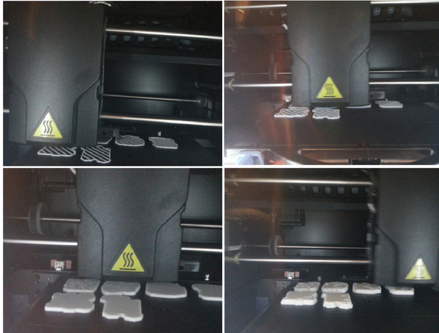
Figure 3. Laying down process of fused ABS polymer in typical FDM equipment.
