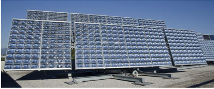
Figure 2. The sun tracker is made of 640 TwinFocus concentrators and has a closed-loop tracking control. Four such trackers have been mounted at the premises of three private companies collaborating to this project. A fourth tracker has been installed by Centro Fermi and the University of Padova. All of them are installed in Northern-East of Italy.
