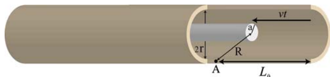
Fig. 1 Artist’s impression of a fiber of radius a, inside a vein of radius r, pulled back with velocity v. “A” is an arbitrary point at the vessel wall at distance R from the centre of the fiber tip. The distance to the fiber tip from a certain position on the vein wall, R(t), which started at position L 0 at t=0, relates to r and distance (L 0 -vt) as R(t) = \sqrt{r^2 + (L_0 - vt)^2}
