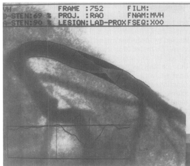
FIGURE 1. Computer output of an analyzed coronary segment. The diameter function is superimposed on the video image; the calibrated diameter values in mm are plotted along the ordinate, and the centerline positions from the proximal to the distal part along the abscissa. The reference position was defined proximal of the stenotic lesion, as indicated in the diameter function by the shaded vertical bar. The central reference position is marked in the artery by a straight line connecting the opposing contour side.
