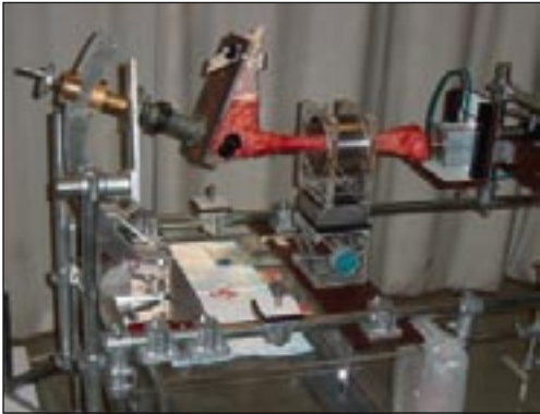
Testing device. The tibia is secured and the foot is attached to a plate, allowing full range of motion (example of maximal dorsiflexion).
