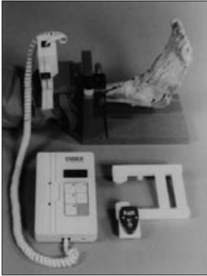
Fig 1. A testing device with a malleolar clamp with two levels and electronic inclinometer is shown.
