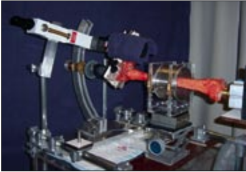
Figure 1. Testing device: the tibia is secured, the foot is attached to a plate, allowing full range of motion, 7.5 Nm external rotation stress is being applied.
