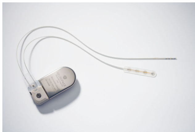
Fig. 2 The RNS Neurostimulator connected to the NeuroPace Depth Lead and NeuroPace Cortical Strip Lead (NeuroPace, Mountain View, CA, USA)
