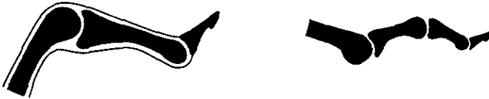
Fig. 4. Biarticular model with two antagonistic tendons.
