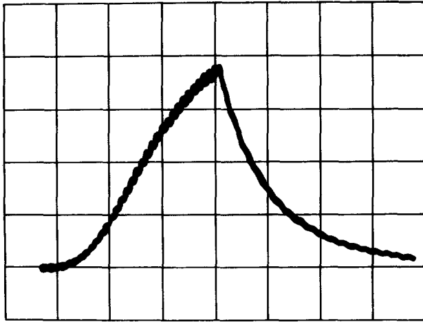
FIGURE 3. Oscilloscopic record of luminance level of a standard stimulus as produced by the halogen light in the perimeters. Horizontal axis: units of 100 msec. Vertical axis: arbitrary luminance units.
