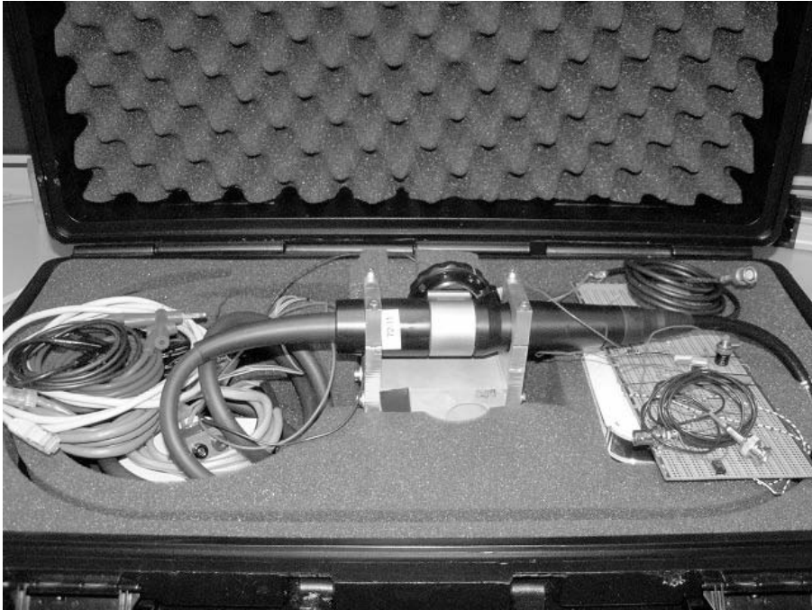
Figure d.1: The first prototype of the fast rotating transoesophageal transducer. Courtesy of Kyriakos Nathanail.
