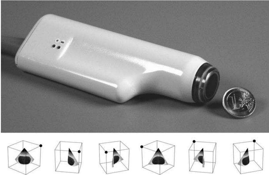
Figure 4.1: Image of the most recent prototype of the continuous, fast-rotating transducer used in this study. Below, a 2D phantom image displayed in perspective from different angles. As shown, continuous rotation results in a curved shape of the original images.
