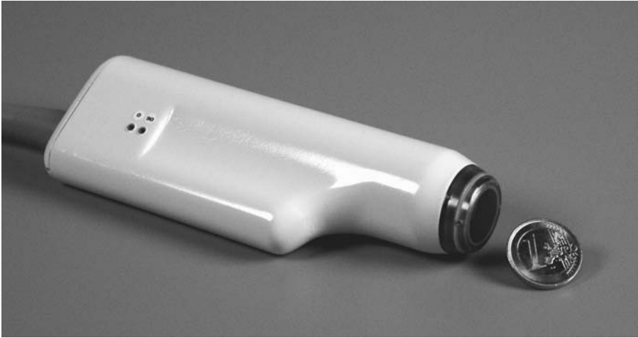
Figure 9.1: Latest prototype of the continuous fast-rotating transducer.
