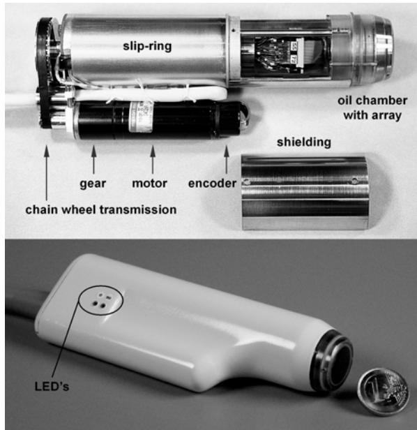
Figure 3.1: The latest prototype of the fast-rotating ultrasound (FRU)-transducer. The upper panel shows the construction of the transducer with some key components annotated. The lower panel shows the transducer with its housing. Note the LEDs on the housing, which are used to indicate whether the phased array is located in one of its two fixed positions ( 0^\circ and 90^\circ ).
