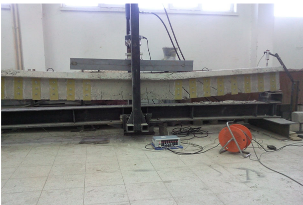
Fig. 7 View of the DE4 specimen after test finished.
