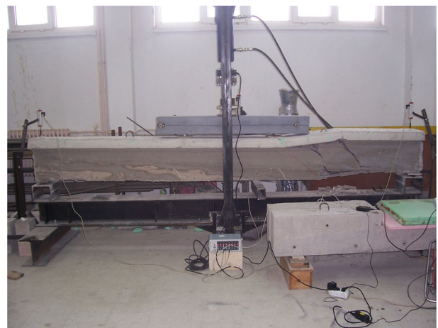
Fig. 5 View of the DE2 specimen after test finished.
