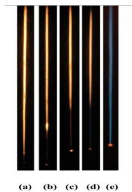
Figure 2.19: Flame streak images of mixtures of diesel and (castor oil) biodiesel:(a) diesel (b) D75B25, (c) D50B50, (d) D25B75, (e) biodiesel [32]
