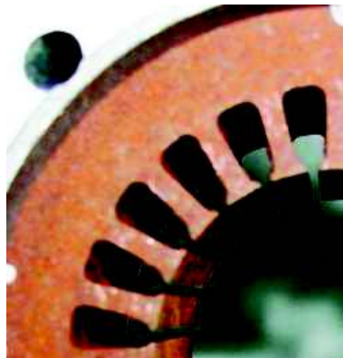
Figure 4.2: Example of semi-closed stator slot.
