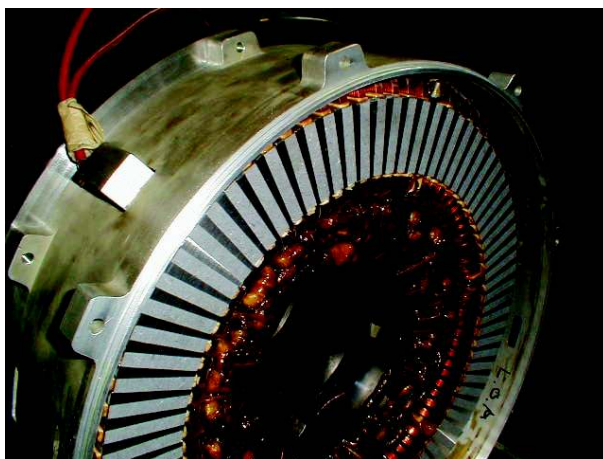
Figure 5.1: Axial flux machine for a in-wheel automotive application. The stator design features flat-turn windings placed in open slots.
