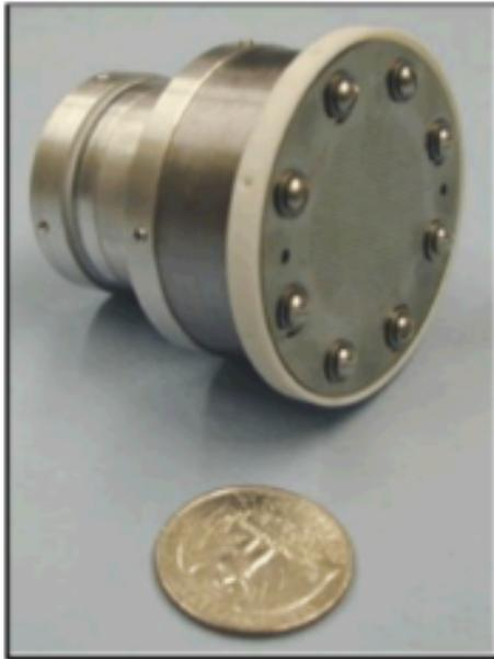
Figure 9. JPL Miniature Xenon Ion Thruster (MiXI) (2).
