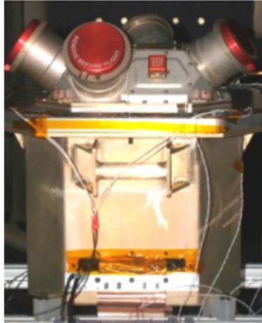
Figure 10. ST-7 Colloid Thruster Cluster (2).
