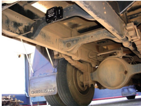
Figure 6. Mounting location of vibration recorder.
