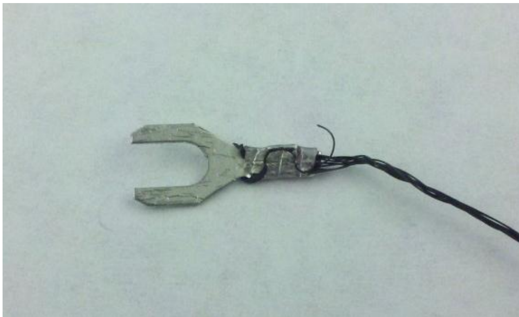
Figure A.10. Nitinol cable with wires wrapped around the end of the spade lug.
