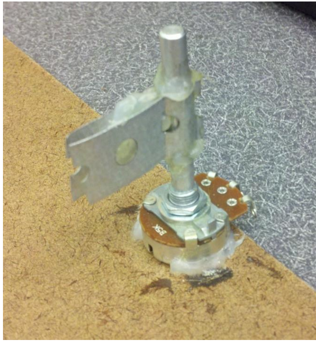
Figure A.5. 5k rotary potentiometer with lever arm used most tests.
