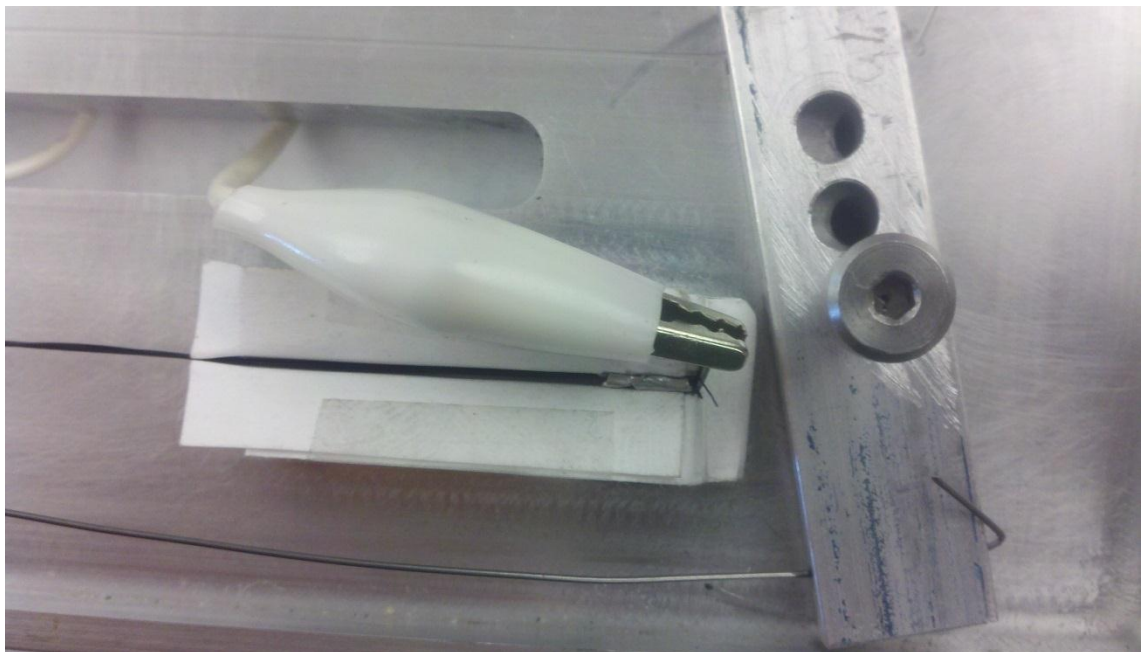
Figure C.6. Nitinol wire attachment to actuator base.
