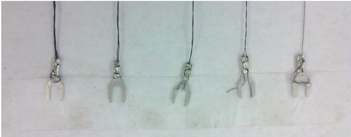
Figure A.8. Nitinol cables of 6 mil diameter wire used for testing.
