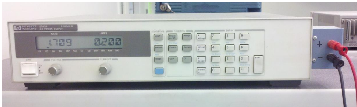
Figure A.1. Constant current power supply used in most tests.
