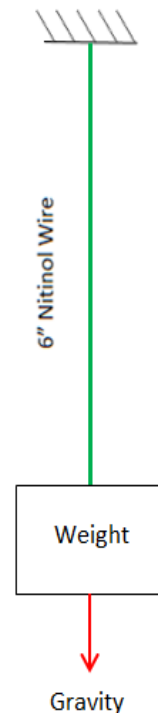
Figure 2.5. Test setup for wire hysteresis test.
