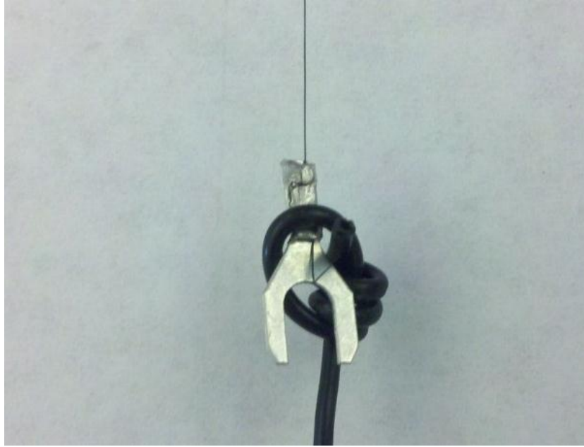
Figure A.17. Weight attachment for wire hysteresis test.
