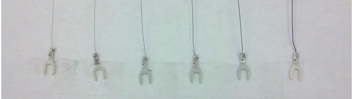
Figure A.7. Nitinol wires used for testing.
