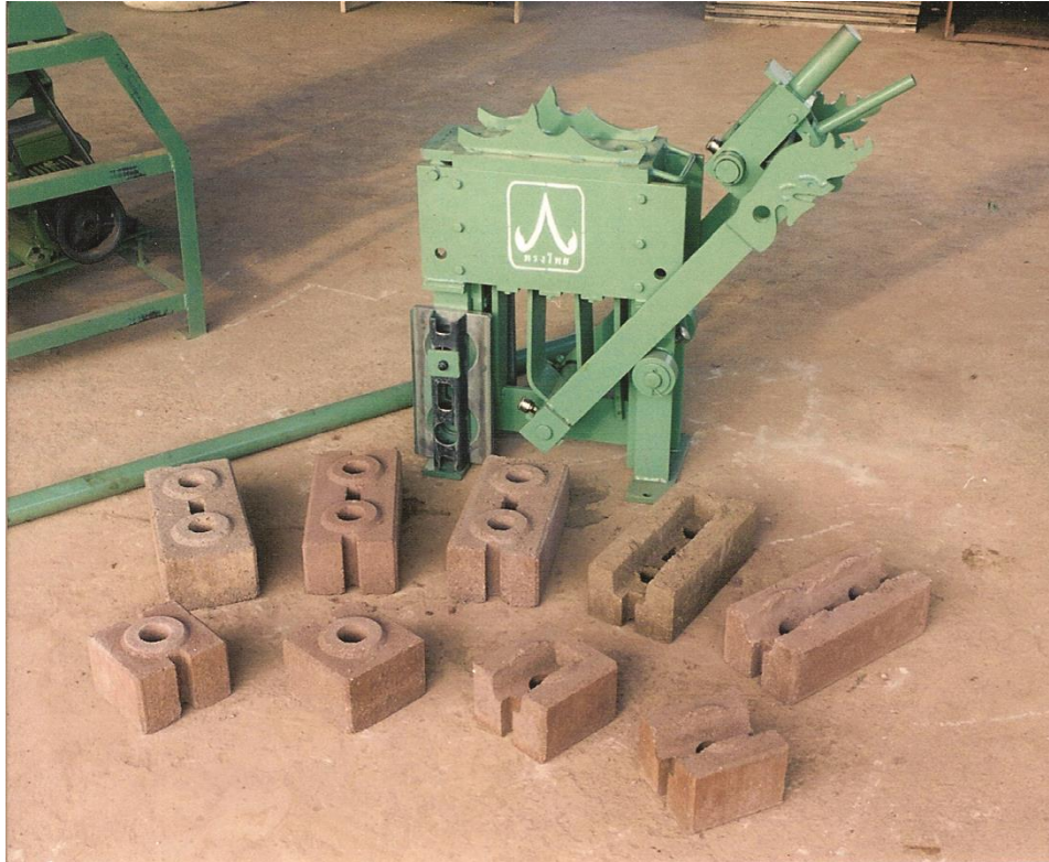
Figure 8: Soeng Thai BP6 block press with 9 different block types (Wheeler 2005)
