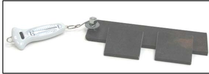
Figure 8. Sled, weights and spring scale.
