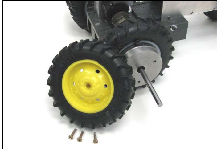
Figure 2. Wheel hub and wheel. Screws go through holes on the wheel into the wheel hub. An Allen screw is located at the top of the hub that fastens the hub to the drive axle.
