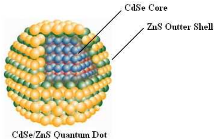
Figure 1 – Illustration of quantum dot showing CdSe core and ZnS outer shell, by Evident Technology [11].
