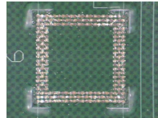
Figure 19. Four UV cured acrylic edge bonds on a board
