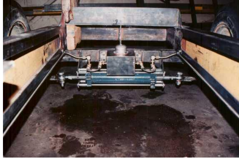
Figure 3. Double acting cylinder steering.
