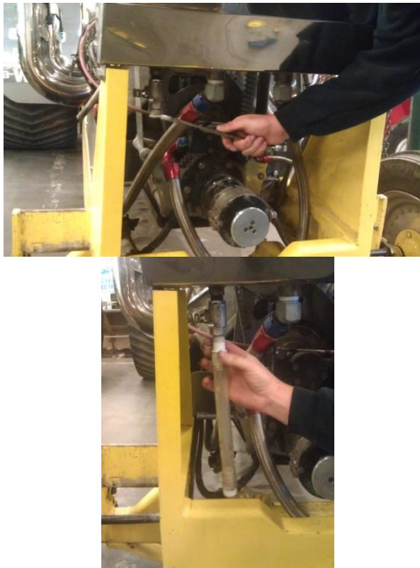
Figure 42. Remove plastic fuel tank plug and attach flexible clear hose.
