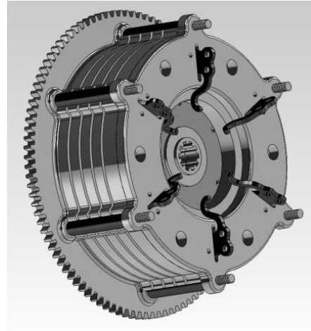
Figure 17: Typical centrifugal clutch on pulling tractors.
