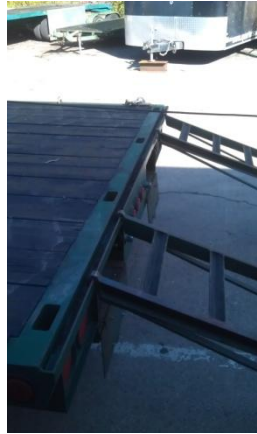
Figure 49. Ramps for single tired trailer.
