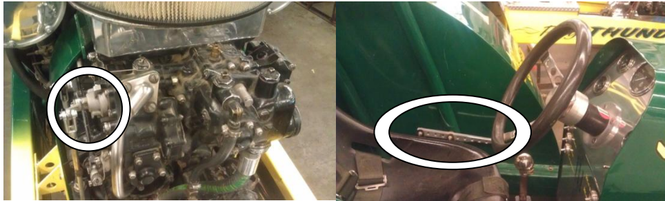
Figure 24. Fuel mixture setting, on carburetor (left), from seat (right).
