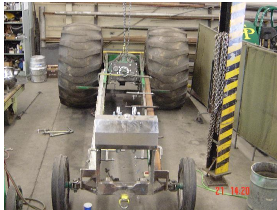
Figure 8. Straightening the frame.
