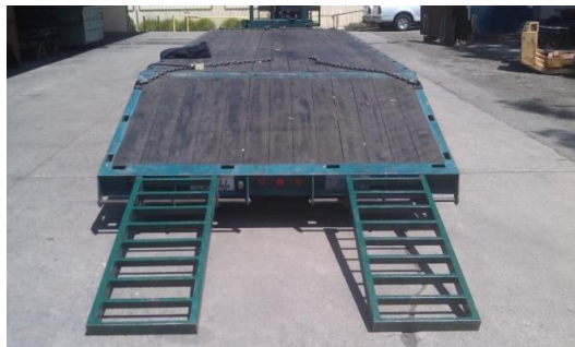
Figure 57. Line up ramps with third board from edge.
