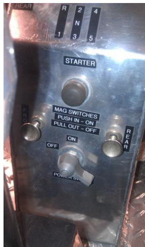
Figure 41. Pull out on the magneto switches to turn them off.
