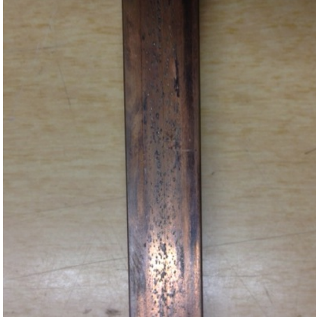
Figure 4: An example of transition damage. Arcing damage seen on the muzzle end of one of the half inch wide Mk 1 rails.
