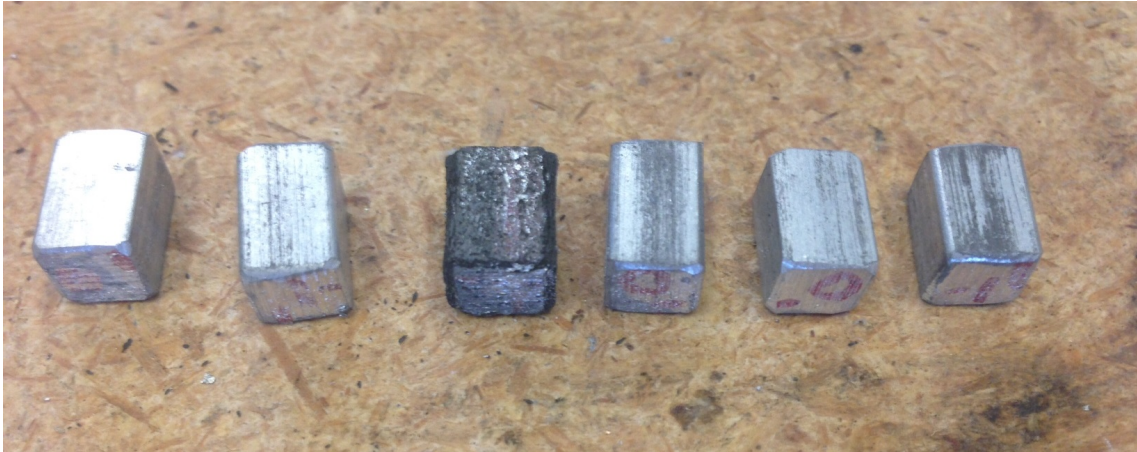
Figure 35: The projectiles a day after being fired on liquid metal coated rails. The heavily corroded projectile was the first one fired and had to push a lot of liquid metal out of the way. The other projectiles show minimal corrosion as dark lines on their contact faces.
