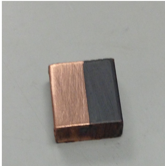
Figure 15: SEM sample one with a graphite coating. The sides of the copper are .5in wide.
