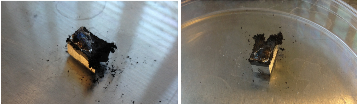
Figure 25: Two views of an Al projectile corroded by eGaIn. The eGaIn can be seen on top, and the black particulate is the corroded aluminum. The corrosion can be seen making its way down the side faces of the projectile. This is the amount of damage after several days.
