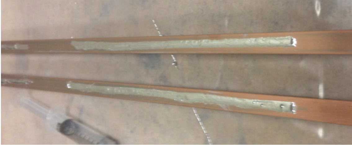
Figure 32: eGaIn applied on the copper rails. The first nine inch segment of eGaIn on the copper rails followed by the plain copper and then finally the beginning of the second seven inch segment.
