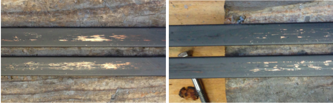
Figure 31: The graphite coated rails after all the static test firings. The places where the projectile dug through the graphite and made contact with the bare copper are seen.
