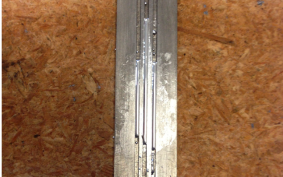
Figure 23: The attempt to wet the liquid metal into the grooved rails. The liquid metal beaded up rather than truly wetting and proved much harder to control.
