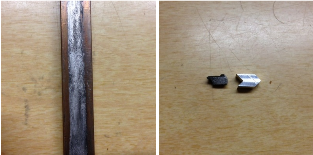
Figure 5: An example of deposition damage. Deposition damage on the breech end of a rail and the resultant mass loss of a projectile.
