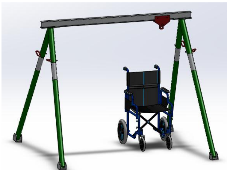
Figure 6-1. Final design of the SideDock frame
