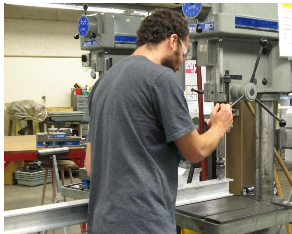
Fig 10-5: Drilling Holes into the overhead beam
