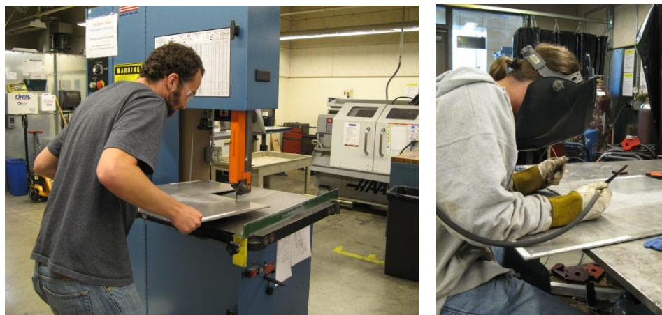
Fig 10-6: Feet Being Cut and Welded
