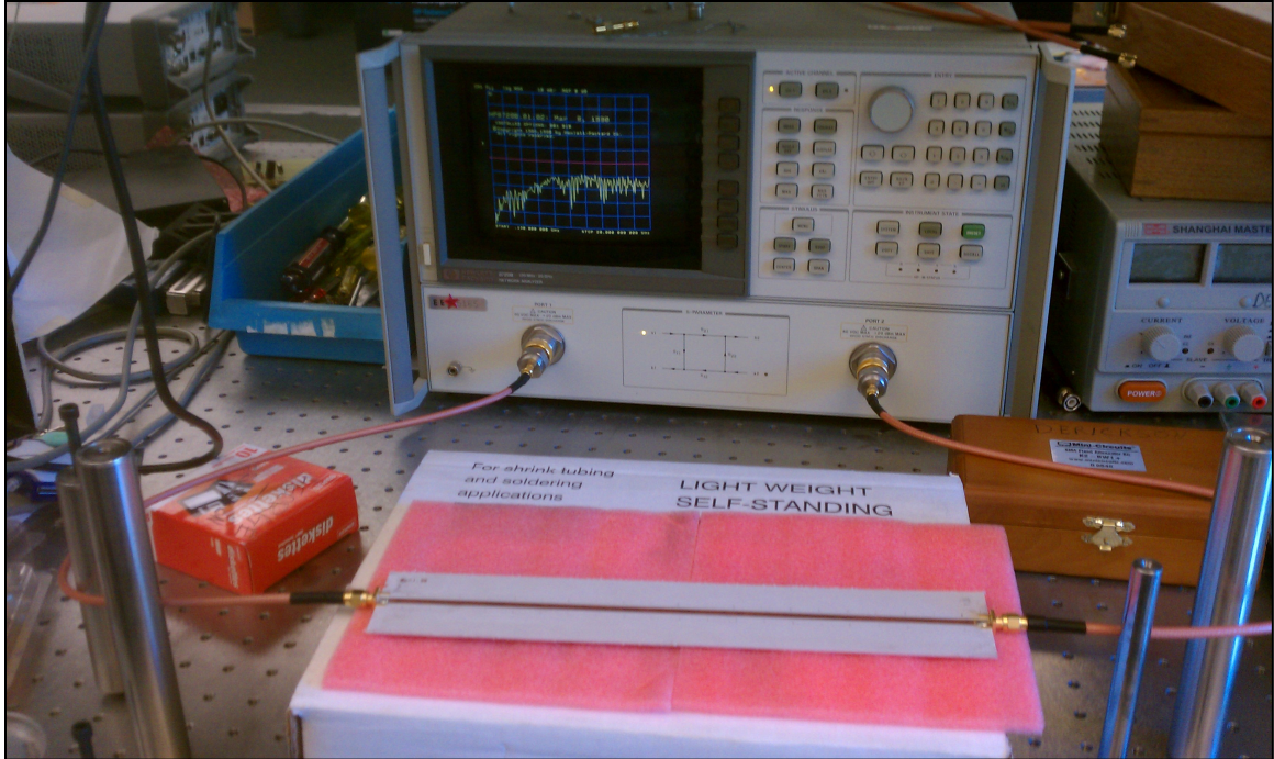
Figure 6.1: HP 8720B network analyzer and microstrip board test setup.
