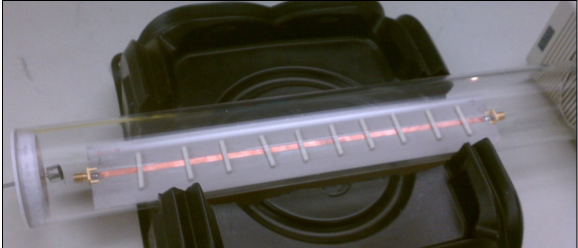
Figure 7.5: Test setup of 1/8" diameter rods on a microstrip board in standing wave tube.
