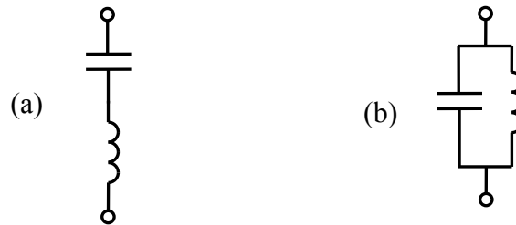
Figure 2.2: (a) Series connected resonant pair. (b) Parallel connected resonant pair.
