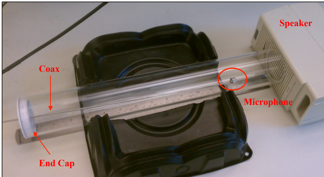
Figure 7.3: Closer view of tube, microphone, coax, end cap, and speaker.
