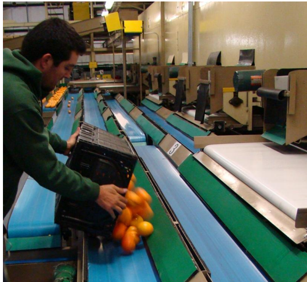
Figure 11. RPC Dump Test by Hand.
