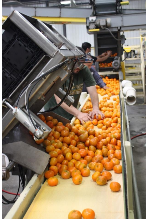
Figure 23. RPC Dumper Test Run.
