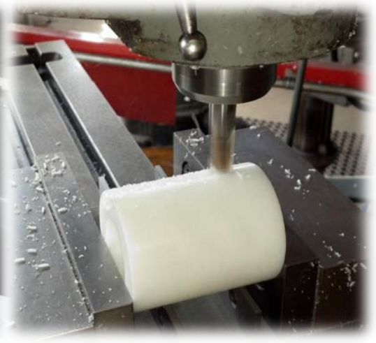
Figure 31. Milling the flat spot on the stick collar that mates with the flat end of the rail collar.
