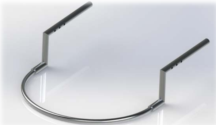
Figure 16. SolidWorks rendering of our final prototype curved rail design.
