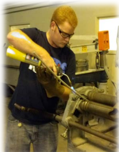
Figure 25. Matt Spaulding heating the curved rail before rolling.
