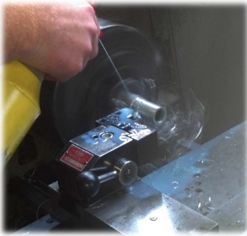
Figure 32. Using a lathe to turn down the outside diameter of the handle portion of the aluminum stick holder. The bike grip can now slide over the handle.
