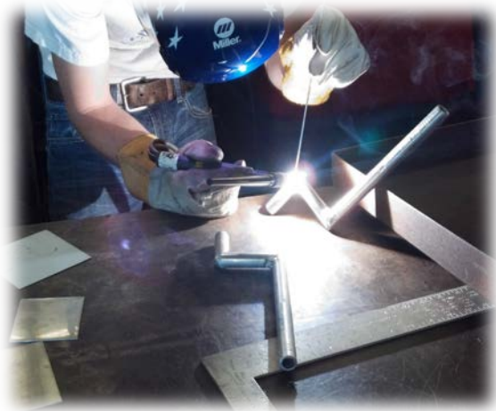
Figure 28. Simon Rowe welding one side of the curved rail support structure together.
