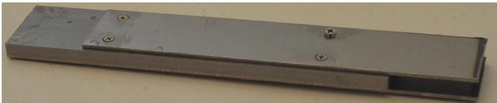
Figure 38: Assembled Pull Test Apparatus
