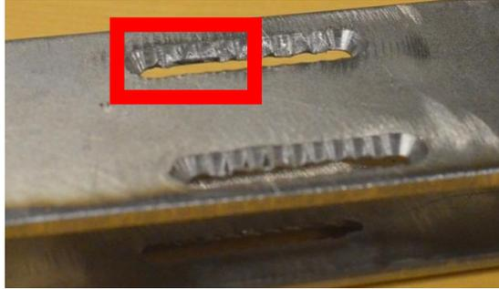
Figure 43: Destroyed Ribs from Pull Test
