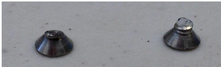
Figure 42: Sheared Screws from 4-Hole Test
