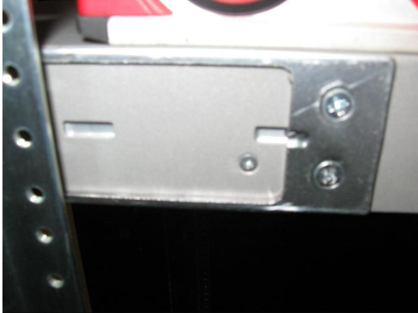
Figure 48: Open Window of Installed Bracket
