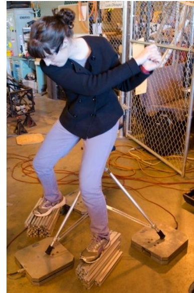
Figure 24: Force Plate Testing of Device
