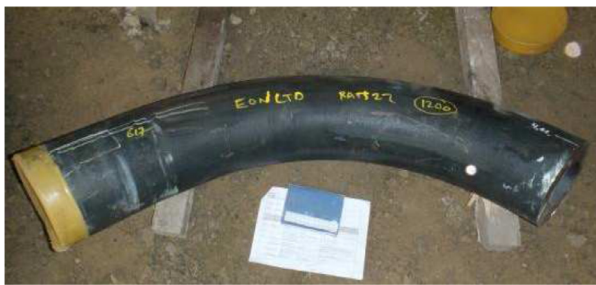
Fig. 3. Section of Alloy 617 piping used for experimentation (shown alongside A4 sheet of paper as size comparison).
