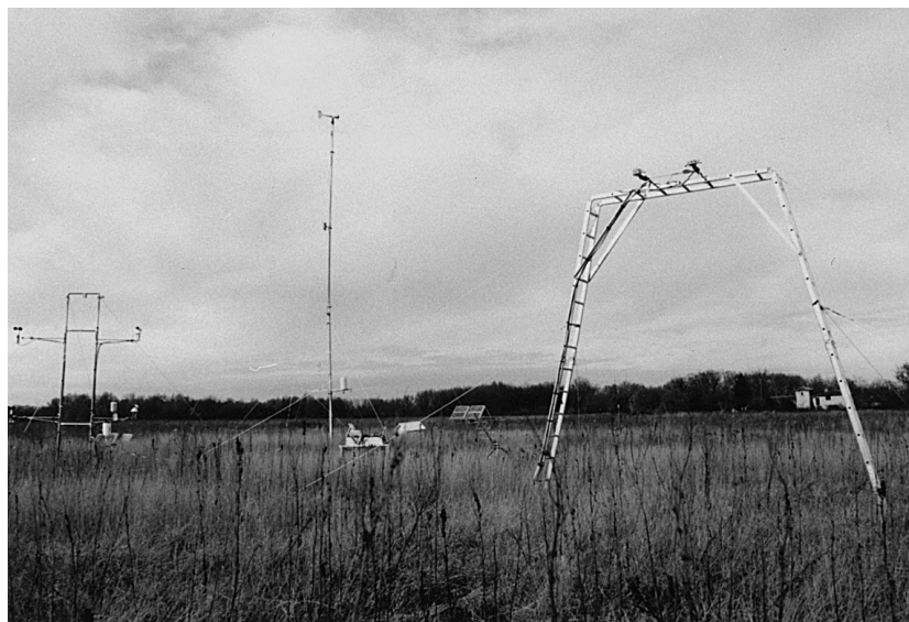
Fig. 1. Photograph of the central part of the MUREX fallow site (at the end of 1996) with some of the instrumentation. From left to right: the two-level SAMER system, the 10-m mast for wind, screen-level temperature and humidity, and IR-temperature, and the scaffolding bearing the radiation sensors
