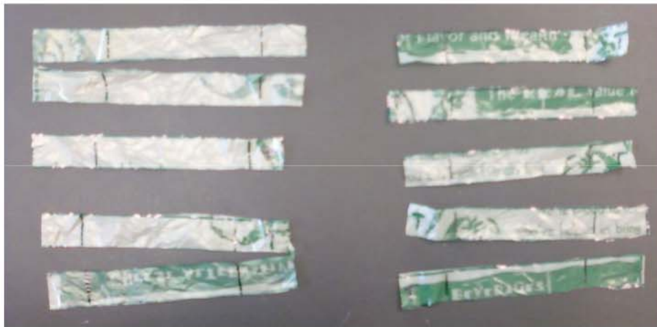
Figure 3: Typical samples marked with a gage length.
