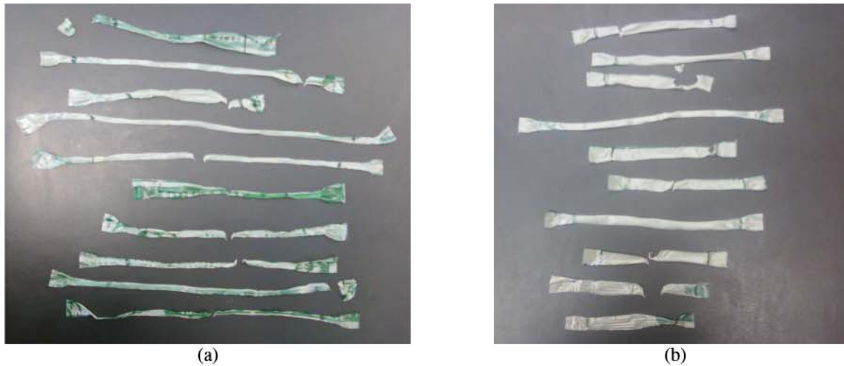
Figure 4: Sample appearance after deformation for (a) Transverse specimens, (b) Longitudinal specimens.
