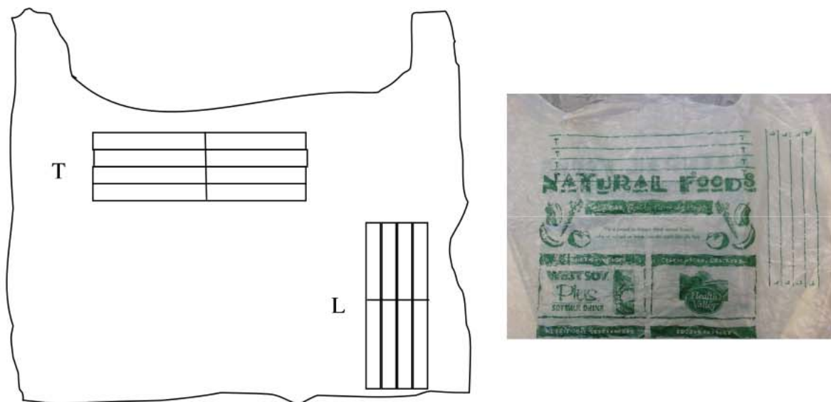
Figure 2: A description of the longitudinal and transverse orientations.
