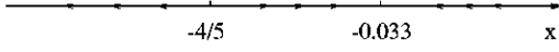
FIG. 3. Renormalization group flow of the ratio of the Lamé coefficients x = \lambda/\mu . The fixed point at x_2 = -0.033 controls the long-scale properties (anomalous elasticity and associated phenomenology) of the pinned spontaneous vortex solid. The critical point at x_1 = -4/5 controls the mechanical instability of the spontaneous vortex solid.
