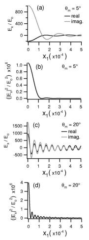
Fig. 6. Plots of the real (black) and imaginary (gray) parts and the modulus squared (black) of the *x* component of the electric field versus  $x_1$  for  $\theta_m$  equal to (a) and (b) 5° and (c) and (d) 20°, respectively. All plots are for  $p_2=10^6$ , n=1.5, and  $y_1=0.$   $z_1$  for each plot is chosen such that the on-axis value of  $|E_x|^2$  is maximum at that  $z_1$ ; i.e., for  $\theta_m=5^\circ$ ,  $z_1=2.997$  and, for  $\theta_m=20^\circ$ ,  $z_1=2.927$ .
