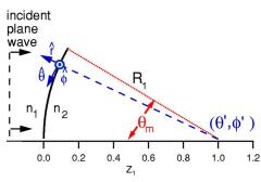
Fig. 1. (Color online) Illustration of the spherical boundary between media 1 and 2; the radius of curvature,  $R_1$ ; the maximum angle of the surface,  $\theta_m$ ; the polar angles to the surface source point,  $\theta'$  and  $\phi'$ ; and the unit vectors  $\hat{r}$ ,  $\hat{\theta}$  and  $\hat{\phi}$ .
