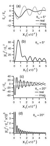
Fig. 7. Plots of the real part (black) and imaginary part (gray) and modulus squared (black) of the normalized longitudinal component,  $E_z/E_0$ , for (a) and (b)  $\theta_m = 5^\circ$  and (c) and (d) 20°, respectively. For each plot  $p_2=10^6$ , n=1.5, and  $y_1=0$ . In each graph,  $z_1$  is chosen such that  $|E_z|^2$  is maximum; i.e., for  $\theta_m = 5^\circ$ ,  $z_1 = 2.997$ , and, for  $\theta_m = 20^\circ$ ,  $z_1 = 2.927$ .
