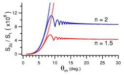
Fig. 2. (Color online) Maximum values of the normalized onaxis irradiance versus the half-angular aperture,  $\theta_m$ , for  $p_2$  equal to  $1 \times 10^6$ . The upper and lower plots are for n = 1.5 and 2, respectively. The dashed curves are calculated using the paraxial approximation, Eq. (52).
