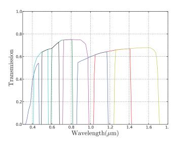
**Fig. 3.** Channel throughputs for the eight channels (five optical and three NIR) assumed in the simulation; the transmissions refer to the telescope + filter + detector combinations.
