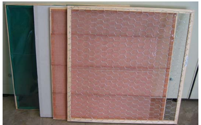
Figure 11. Environmental barriers simulated actual wireless-system environments: (l-r) ESD, drywall, copper mesh, and poultry-net barriers.
