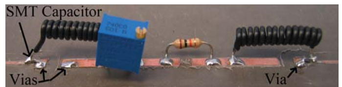
Figure 25. The amplifier's bias circuit.
