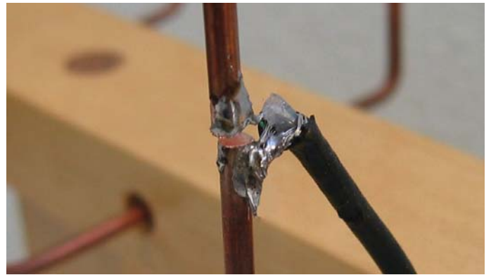
Figure 20. The Quagi was fed on the vertical side by a coaxial cable. The gap length was 1/32 in.
