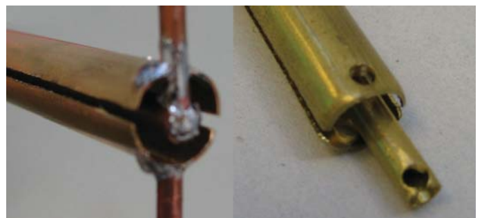
Figure 12. The corner reflector dipole's input matching.
