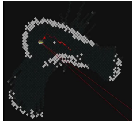
Figure 7. Example of a map created from implementing FastSLAM while in motion.
