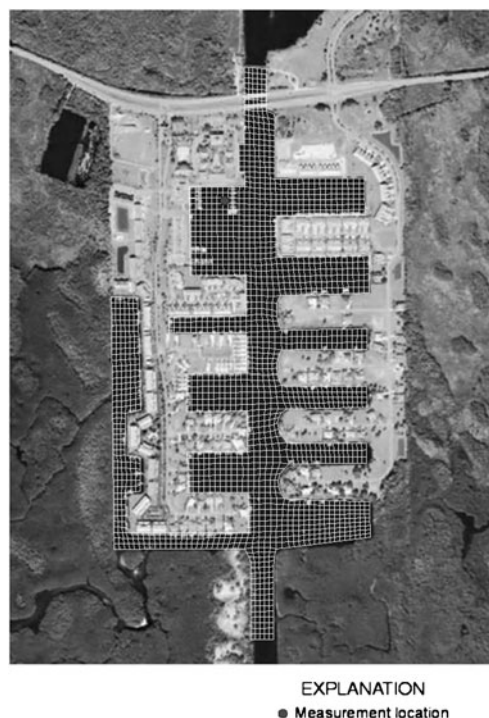
Fig. 3 Map of Port of the Islands showing grid for three-dimensional hydrology model application. North end of grid is a tidal-blocking weir. Major east–west road is U.S. 41
