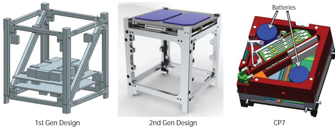
Figure 2. CAD Renderings of different PolySat satellites. The CP7 rendering illustrates how mission-specific batteries were utilized in the payload bay.
