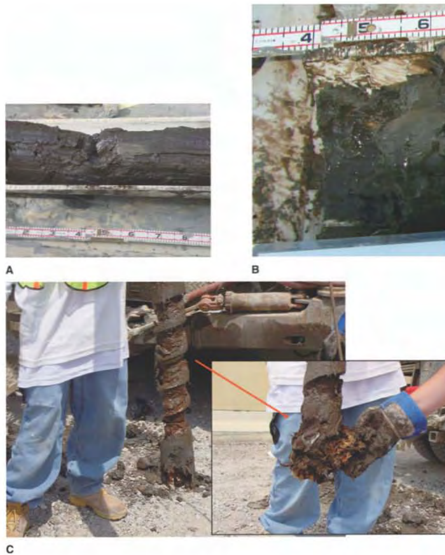
Fig. 14. (Color) (a) Sheared sample of the sensitive organic silty clay layer from within the slide area; (b) unsheared sample of the same material from near to the slide area, but not within it; and (c) shiny dark brown to black sensitive organic clay on auger stem and (inset) closeup view of layers of leaves and twigs—17th Street Canal breach site
