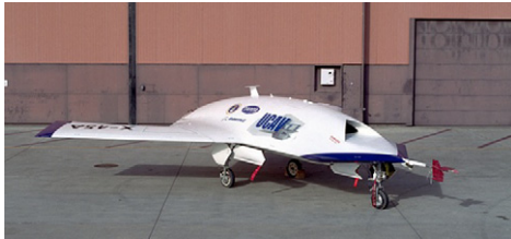
Fig. 3. X-45A UCAV configuration (photo courtesy of NASA Dryden Flight Research Center).
