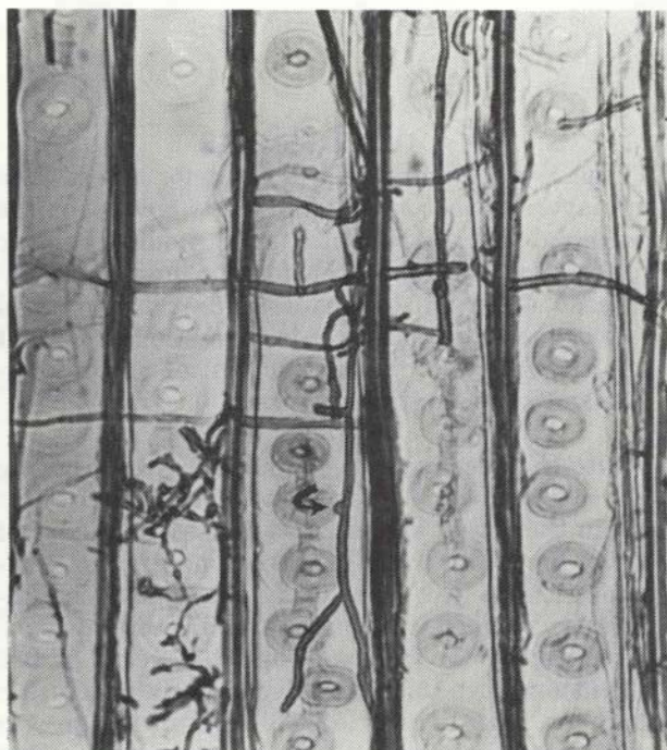
Figure 8. Early to moderate stage of decay (estimated 15 to 25 percent weight loss) in discolored giant sequoia heartwood associated with carpenter ant galleries from the failure zone of a stem failure (Specimen L-1) in the Lost Grove area. Note hyphae, one of which has a clamp connection (→). (Magnification 320 X)
