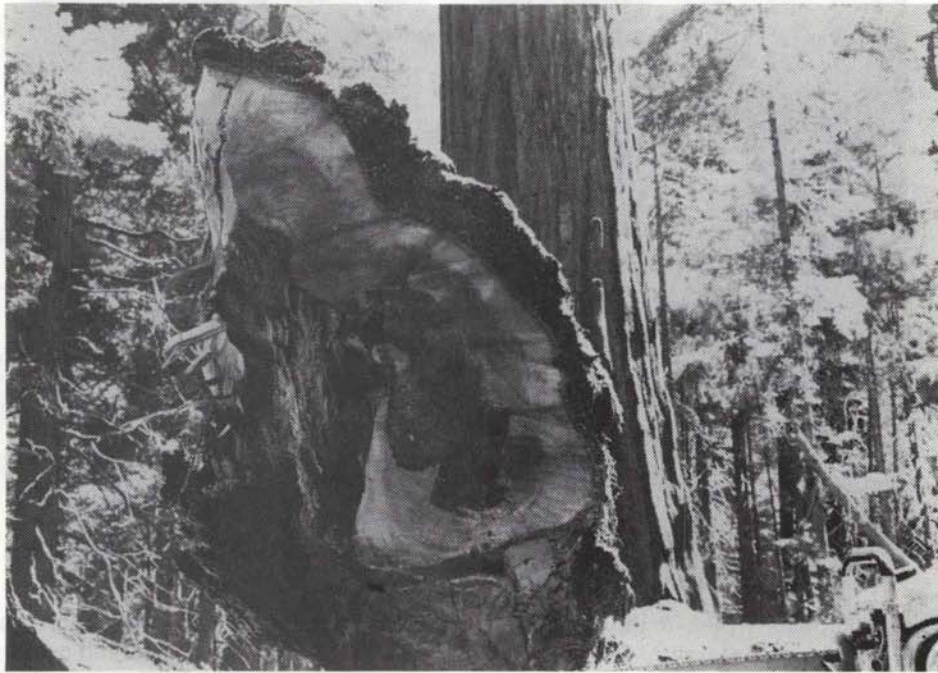
Figure 5. Sectional view of a root from a root failure (Specimen W-4) in Whitaker's Forest adjacent to Sequoia-Kings Canyon National Park. Note the advanced decay (stringy rot) on the left side of the root.
