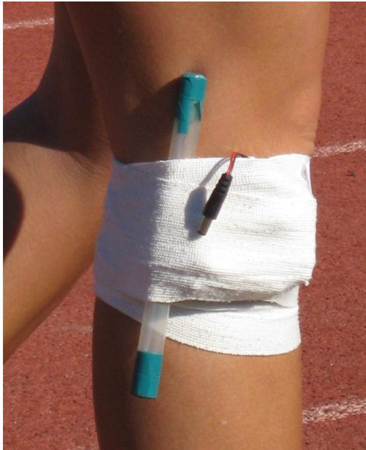
Figure 8: Device wrapped on the upper part of the calf with vertical orientation
