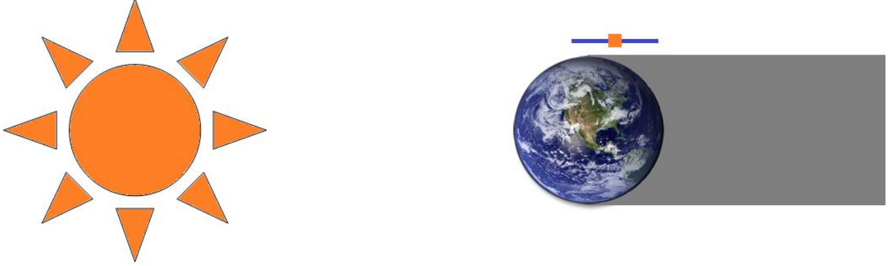
Figure 4. Absence of a line of sight between a spacecraft and the Sun shown as darkness.
