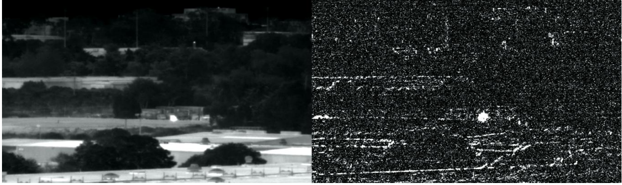
Figure 6: Original Midwave IR Image on the left, and Absolute Difference Image on the right
