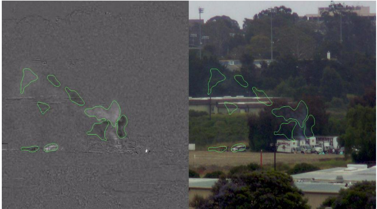
Figure 45: Superimposed Mask using Adaptive Threshold over both Respective PC2 and RGB Image
