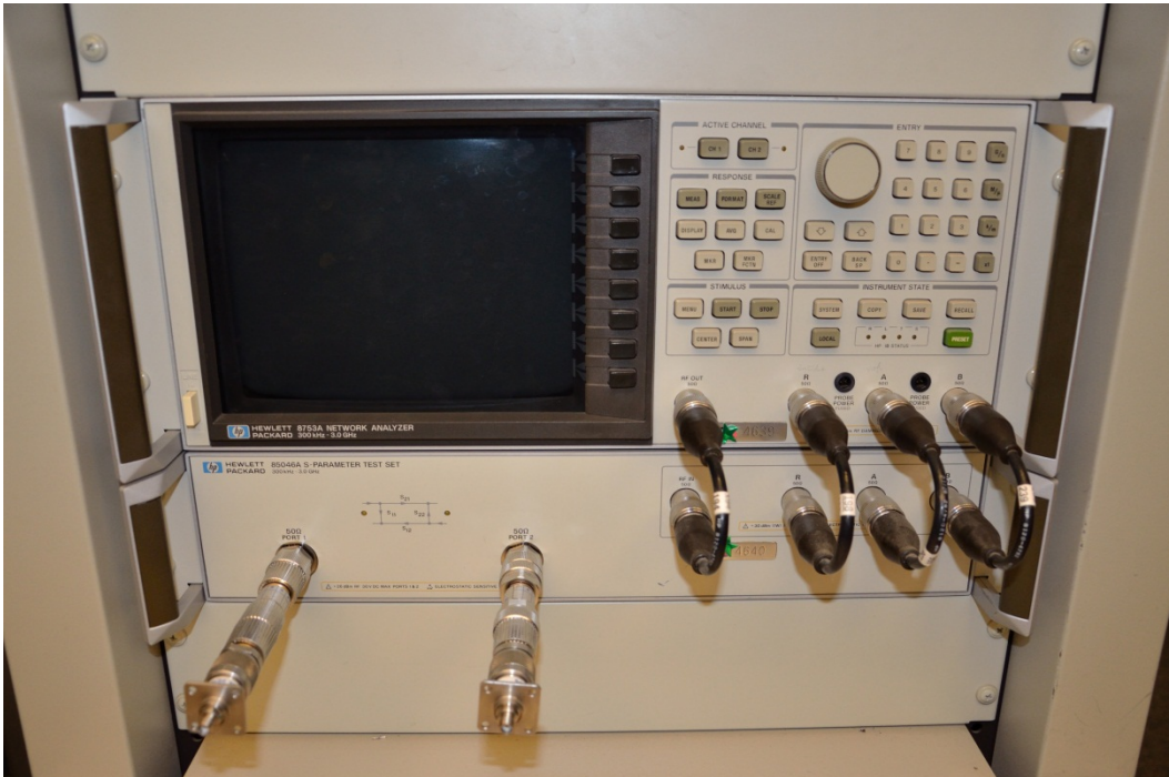
Figure 4.7 HP8753A VNA used to measure inductors, capacitors, and impedance responses of the bias choke and output network.
