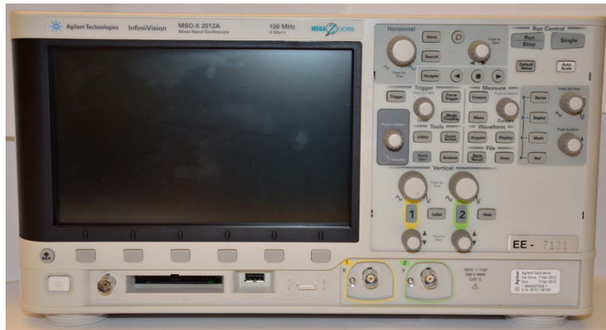
Figure 4.20 The Agilent MSO-X 2012A function generator/oscilloscope used as the RF source to the PA and used to view waveforms on the prototype.
