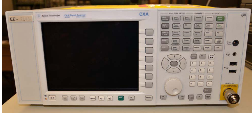
Figure 4.22 The Agilent CXA N9000A spectrum analyzer used perform spectral analysis on the class C PA.
